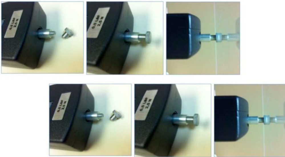
FIG. 3 Attaching the Force Gauge to Spray Disc
